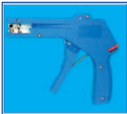
SA83 Tie strap installation gun, tightens and then cuts the tie wrap
